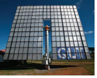
A concentrated photovoltaic (CPV) system being tested in a joint QUT and Sumitomo Electric Industries project at the Queensland Government's Redlands Research Facility.
